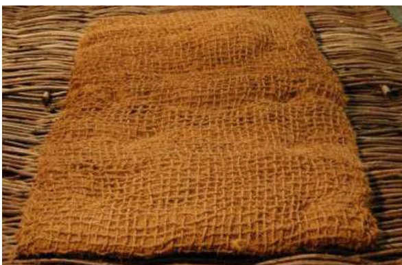
3.9 (b) Cooler Mat from Coir
