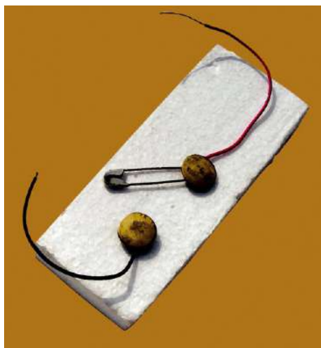
Figure 12.12 An Electric switch
