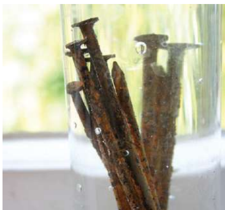
Fig. 6.5 Rusting of iron nails
