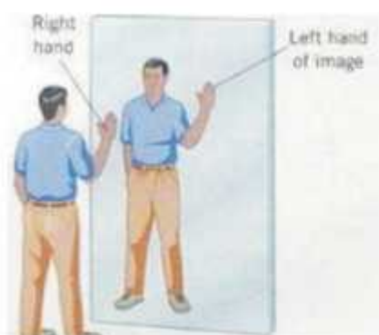
Figure 15.6 (a): Lateral Inversion of hands of a person by plane mirror.
