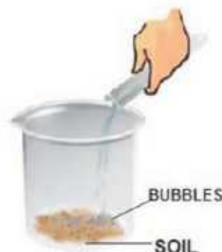
Fig 9.11 Testing the presence of air in soil
