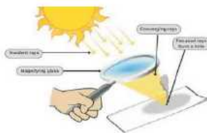
Figure 15.15 (b): Image of Sun by using a convex lens.
