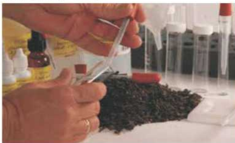
Fig 9.6 Testing the pH of soil
