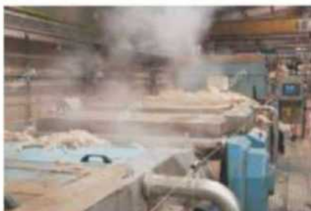
Fig 3.8 (b) Scouring by machines
