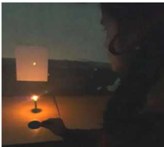
Figure 15.11: Image of an object on screen formed by a concave mirror
